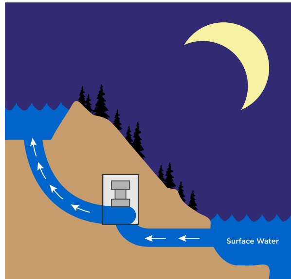
Water is pumped uphill to the reservoir for use the next day.
